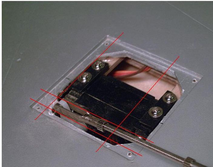
Remove the linkage from the servo arm, and rotate the arm below the level of the servo cover. Install the servo cover (illustrated in black below). Using the lines around the outside of the cutout, draw the extents of the required cutout as shown below.
