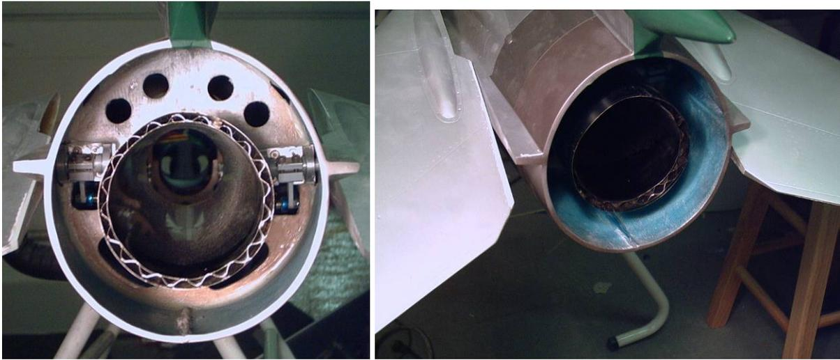
Apply several couple of coats of BVM Heat Shield to the aft area of the bypass. The upper portion of the bypass, if used, may be trimmed to suit the particular turbine installed and retained with Velcro straps.
