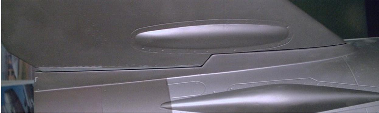
Cut away the vertical face of the notch at the fuselage root as shown below to allow the H-stab to rotate. This area is covered by the stab so it's not visible when the stabs are at neutral.
