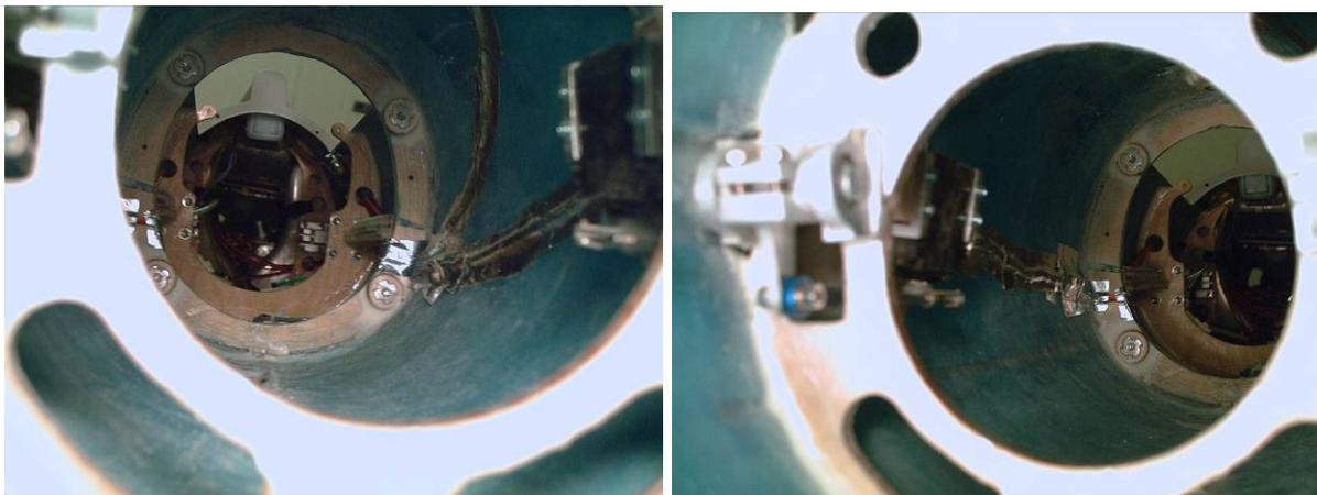
The aileron and flap servo wires are routed from the cutout in the wing root forward over the cutout for the gear strut. This area can become easily congested as several pneumatic lines route through this area. Ensure that the air lines and servo wires are routed such that they are not chaffed by the main wheels when the landing gear is retracted.
