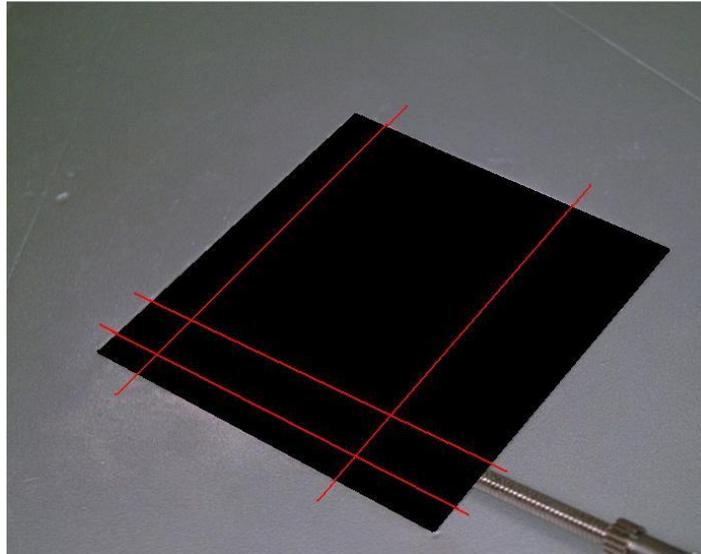
Drill a hole at each end of the slot such that the drill diameter is the same as the width of the slot. Using a knife, saw, or cutoff wheel, remove the remaining slot material (colored in red in the photo below). Screw the servo cover into place and reattach the linkage to the servo arm. Check that the servo arm and linkage does not bind on the cutout. Trim/sand the edges of the slot as required.
