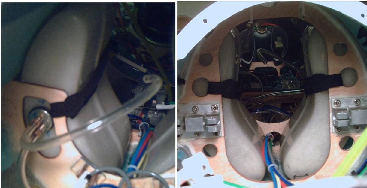
The main fuel tank is supported at the rear by the saddle tanks. A front support can be made from 1/8" plywood screwed to hardwood blocks Hysol'd to the fuselage. Adhesive-backed Velcro applied to the tank and support can be used to secure the tank from moving forward/aft.
