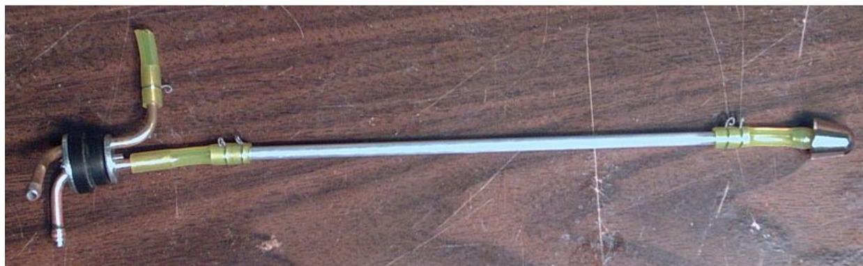
The forward face of the main tank, when installed in the model is quite close to the rear face of the cockpit. As such, a 90 degree bend in the fuel and vent lines prevents any interference between the lines and the cockpit.
