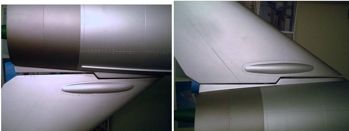
Portions of the root chord may be sanded down or build up using spot putty, as required, to adjust the H-stab root contour such that it matches the fuselage. This will allow the stabs to be installed with only a 1/32" gap between the stab and the fuselage which will enhance the look of your model. Use touchup paint to blend any spot putty visible. See "After" photos below.
